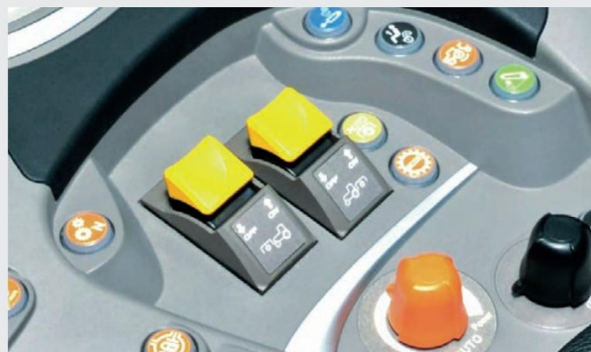
↑ PTO adjustment and activation are conveniently integrated into the armrest ...
