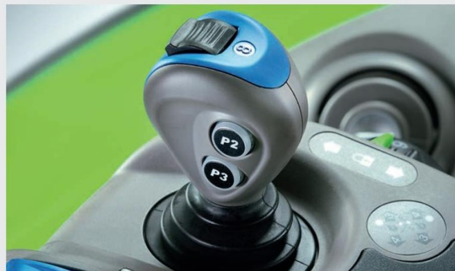
↑ The cross-control lever with rocker switch controls three hydraulic control valves.
